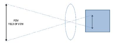
• Focal Length. This is the distance from the lens to the camera's imager. It is always specified in millimeters. Focal length determines the relationship between working distance and angle of view. In other words; how big of an area you can see at a given distance.
