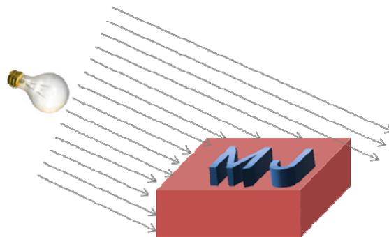
**3-Back Light** - This method provides a good outline of the part to be inspected. This can be used for shape verification and dimensional measurements.
